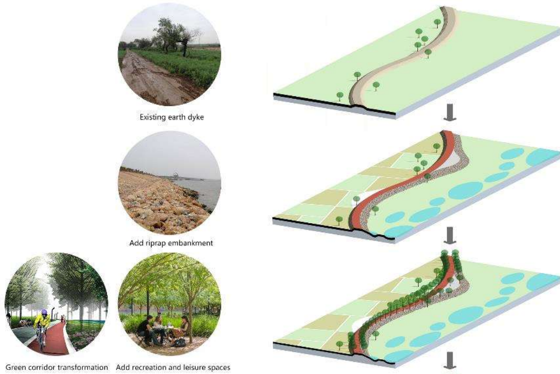
Image 20: change existing earth dyke into the central green corridor
